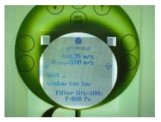
The panel displays "Wait" until the velocity is OK. Then, the panel displays "Flow Correct" and you can work.
