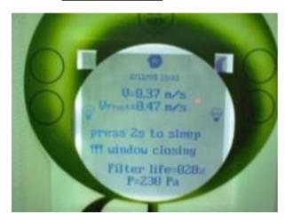
Push Sleep switch during 2 seconds to turn on the cabinet in stand by mode. When the moon is highlighted, it's OK.
