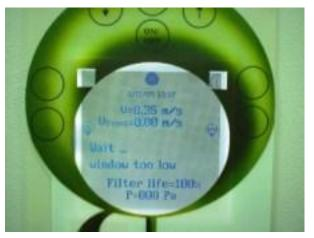
The panel displays "Wait" and the sash window stays closed until the velocity is OK. Then, the window raises itself to the correct height.
