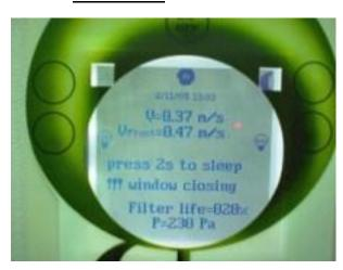
Push Sleep Button during 2 seconds to switch the cabinet in Sleep mode. When the moon is highlighted, it's OK.
