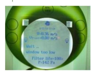
When the cabinet comes back to the normal use, the sash window stays closed until the velocity is OK. Then, the window raises itself to the correct height.
