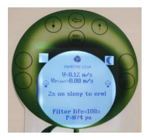
To switch from standby mode to working mode, press the button of for 2 seconds until the moon becomes clear. As soon as the hood returns to normal mode, the message "correct flow" is displayed.
