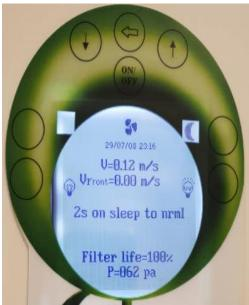
When the UV lamp is on, small rays appear on the screen logo. The UV lamp switches off automatically after the programmed duration (factory setting: 30 minutes). Can be modified in the "UV duration" section of the user menu.
