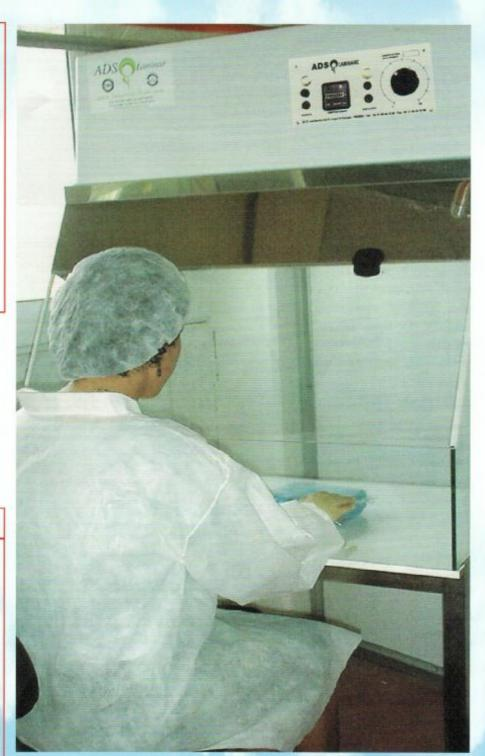
UNIVERS MAV can be installed on its own stand INTERNAL DIMENSIONS 905 x 600 (depth) x 700 (height)
