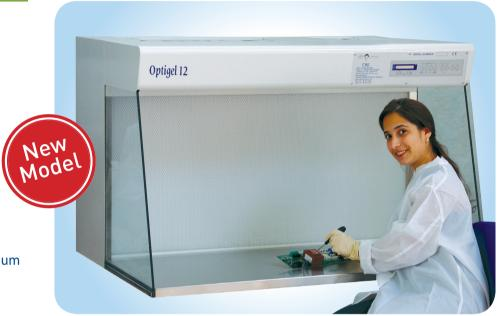
The new OPTIGEL provides a clean air working area of Class ISO-5, according to ISO-14644. Air constantly flows horizontally through an absolute HEPA filter into the working area, thus protecting the product inside the cabinet from existing particles in the air.
