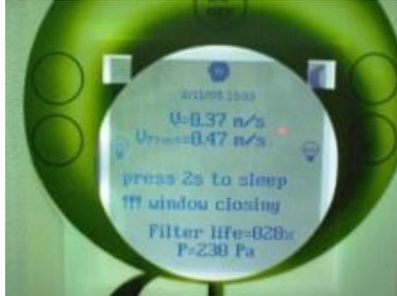
Then, the window closes automatically (an alert message displays) and the light switches off. It is possible to switch ON the light if necessary.
