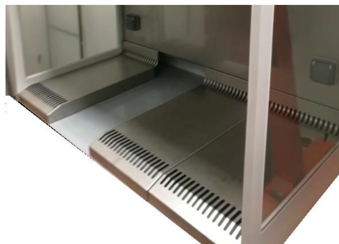
Split work surface / air barrier
